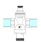
The pressure reducers MINIBRASS don't get the effects, in their functioning, of gravity force; therefore they can be installed in the plant in any position:
