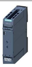
TIME RELAY, ELECTRONIC, DELAYED, 2 CO CONT., 15 TIME SET. RANGES, 0.05S...100HR, 12...240V AC/DC AT AC 50/60HZ LED, SPRING-LOADED TERMINAL (PUSH-IN)
