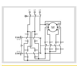
For single-speed reversing motors 30205087 (4NO) contact block
