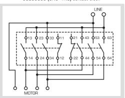
For two-speed reversing motors 30205086 contact block
