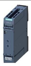
TIMING RELAY, ELECTRONIC, OFF-DELAY, WITHOUT CONTROL SIGNAL OR NON-VOLATILE RELAY DEFINITE PASSING MAKE CONTACT, 7 T. SET. RANGES 0.05S...600S, 24 V AC/DC, 1 CO CONTACT W. LED, SPRING-TYPE (PUSH-IN) TERMINAL
