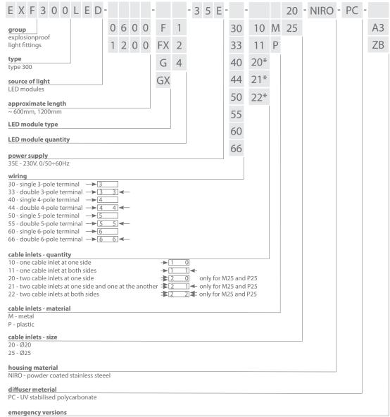
A3 - version with 3h emergency power module available only with 34E power supply (250V, 50-60Hz). Works in the temperature above 0°C. Configuration 11P20 is NOT available for the emergency version 0600-..-A3
