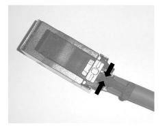
Press down on lid to fully terminate wires onto IDC terminations. Ensure the bunched cable fits neatly between pillar guides to prevent trapping of wires and or foils.
