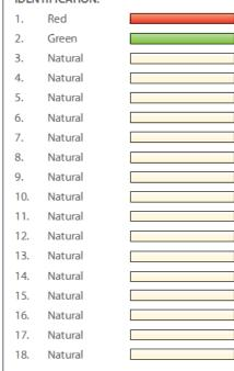
Note: Where fillers are present in a loose tube design, these will be used as markers and coloured accordingly.
