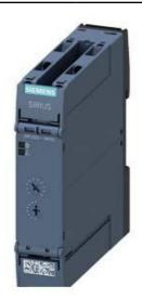
TIME RELAY, ELECTRONIC, DELAYED, 2 CO CONT., 15 TIME SET. RANGES, 0.05S...100HR, 12...240V AC/DC AT AC 50/60HZ, SCREW TERMINAL
