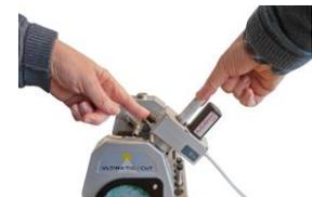
**Important:** The locking pin must not be held down, when the AutoGrind is started or pressed down during grinding. This will destroy the inner parts of the module!
