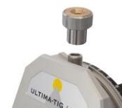
The included stretching screw (Item No. 44550022) must be mounted in the angle adjustment unit, using a little bit of white grease on the thread, and firmly tightened with a 14 mm wrench. The included tightening screw (Item No. 75550019) is mounted loosely on the stretching screw. Then the desired grinding angle is chosen and the tightening screw is tightened firmly by hand.
