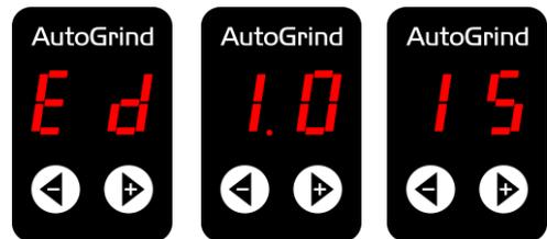
The grinding time (see section #7, iii) can be adjusted from 1 to 99 sec. The adjustment is done by pressing the “+” and “-” buttons on the front of the controlbox. Each push changes the grinding time with 1 sec.
