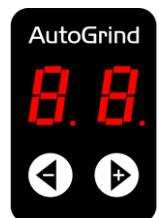
If the power is disconnected for 5 sec. the controlbox returns to the grinding program.
