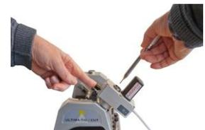
The electrode holder should be rotated with a light pressure until the electrode holder locks into the drive unit, you will feel a slight click as the electrode holder is in position. Next push the electrode holder in and rotate counter-clockwise until the bayonet lock is holding the electrode holder in place.
