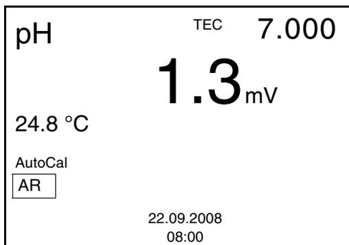
12 | Wait for the measurement with stability control to be completed or terminate the stability control and take over the calibration value with **<ENTER>**.
