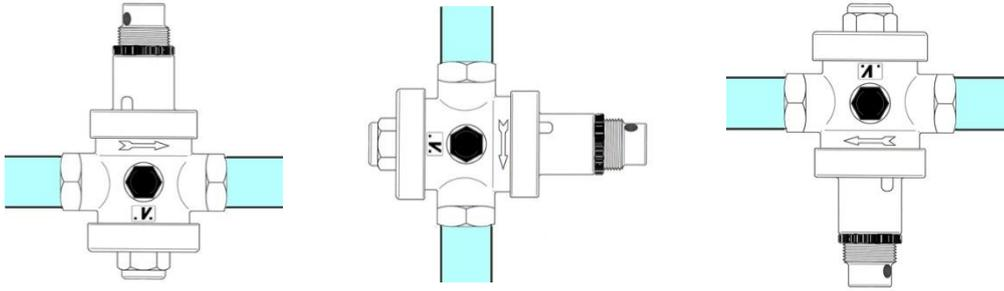
The pressure reducers EUROBRASS 143 don't get the effects, in their functioning, of gravity force; therefore they can be installed in the plant in any position:
