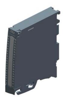
SIMATIC S7-1500, DIGITAL INPUT MODULE, DI32 X DC24V, 32 CHANNELS IN GROUPS OF 16; INPUT DELAY TYP. 3.2MS; INPUT TYPE 3 (IEC 61131) INCL. FRONT CONNECTOR PUSH-IN
