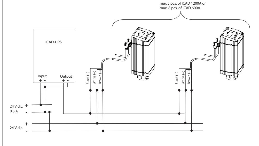
One 24 V DC transformer for ICAD-UPS and ICAD 600A / 1200A
