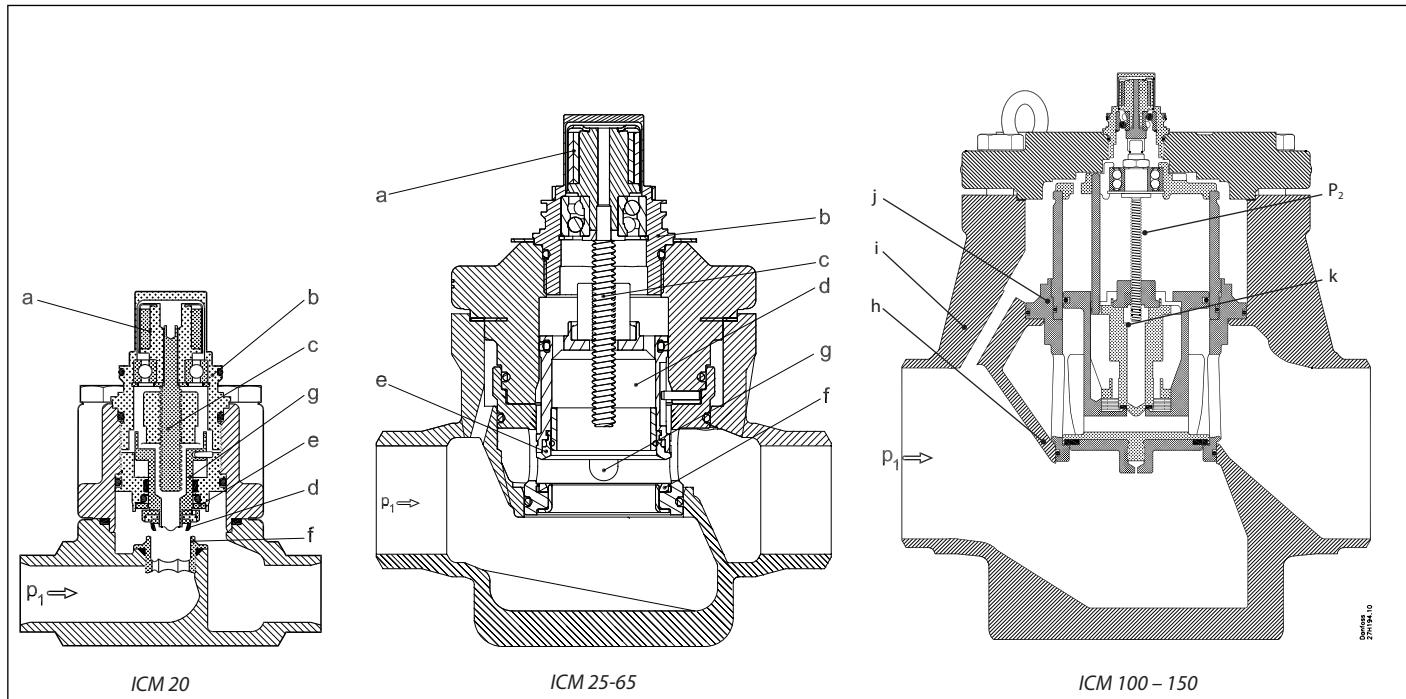
**ICM** motor operated valves are designed for use with the **ICAD**, Industrial Control Actuator with Display.
