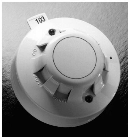
The Intellia ionisation detector EDI-10 uses a low activity radioactive foil to detect fires by irradiating the air in the smoke chambers and causing a current
