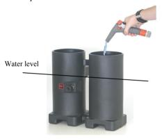
15. Replace the depressurising foam and lid and place the test bottle in it's location on top of the lid.
