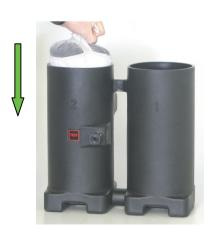
10. Connect the inlet to the condensate collection pipe.
