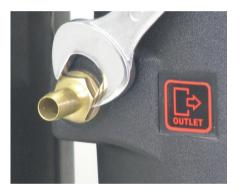
6. Screw the inlet nipple with rubber o-ring in to it's marked location using a 22 mm wrench
