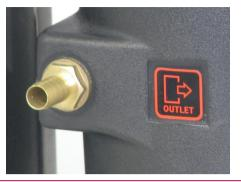
13. Fill the unit with water from tower 1 until both towers are filled and water flows out of the outlet point.
