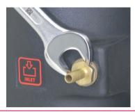
8. Screw the test drain with o-ring in to it's marked location using a 17 mm wrench.
