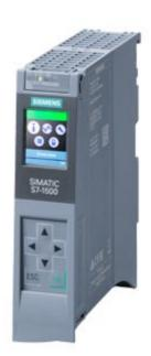
SIMATIC S7-1500F, CPU 1511F-1 PN, CENTRAL PROCESSING UNIT WITH WITH WORKING MEMORY 225 KB FOR PROGRAM AND 1 MB FOR DATA, 1. INTERFACE: PROFINET IRT WITH 2 PORT SWITCH, 60 NS BIT-PERFORMANCE, SIMATIC MEMORY CARD NECESSARY
