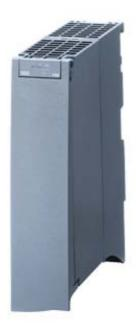
SIPLUS S7-1500, CM PTP RS422/485 BA COMMUNICATION MODULE FOR SERIAL CONNECTION RS422, RS485 FREEPORT, 3964(R), USS, 19200 KBIT/S, 15-PIN SUB-D FEMALE CONNECTOR -40 ... +70 DEGREE C WITH CONFORMAL COATING BASED ON 6ES7540-1AB00-0AA0
