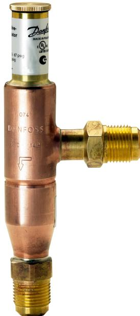
KVC hot gas bypass regulator are used to adapt compressor capacity to actual evaporator load by supplying a replacement capacity in form of hot / cool gas.
