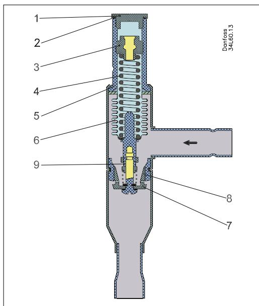
Hot gas bypass regulator type KVC opens on a fall in pressure on the outlet side, i.e. when the pressure in the evaporator reaches the set value.
