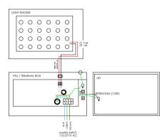
Wire the Mains cable into the terminal block. Provision has been made for this and identified as the E (Earth), L1 (Switched Live), L2 (permanent live) and N (Neutral) terminals. There are two pairs of contacts for each of these to facilitate a mains cable that can be looped in and out of the unit. The L2 terminals on a standard unit are not electrically connected but allows them to be used on the same circuits as *emergency units*.
