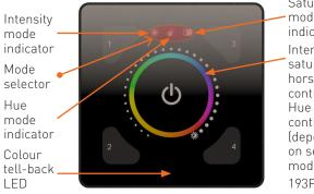
Saturation mode indicator Intensity and saturation horseshoe control / Hue (colour) control circle (depending on selected mode) 193PB
