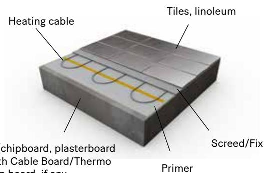
Existing floors (chipboard, plasterboard or concrete) with Cable Board/Thermo Board insulation board, if any. On EPS concrete/cement, reinforcement mesh is required. When laying on reinforcement mesh, the cable must be laid on the top of the reinforcement mesh.
