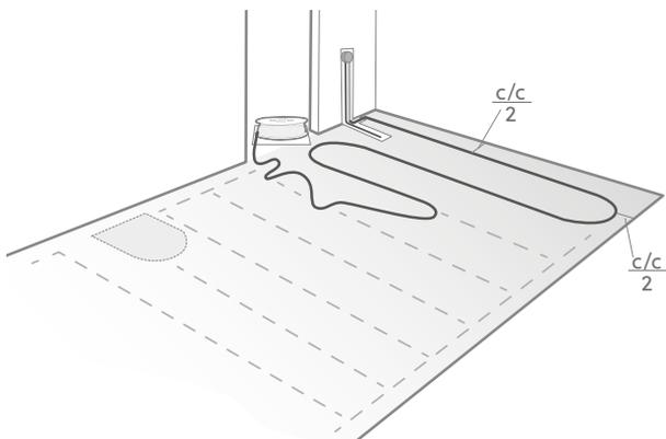
4. This is how the heating cable should be laid around floor drains and similar. Leave space for the floor drain grille. NB! At least 20 cm distance between drain and heating cable!
