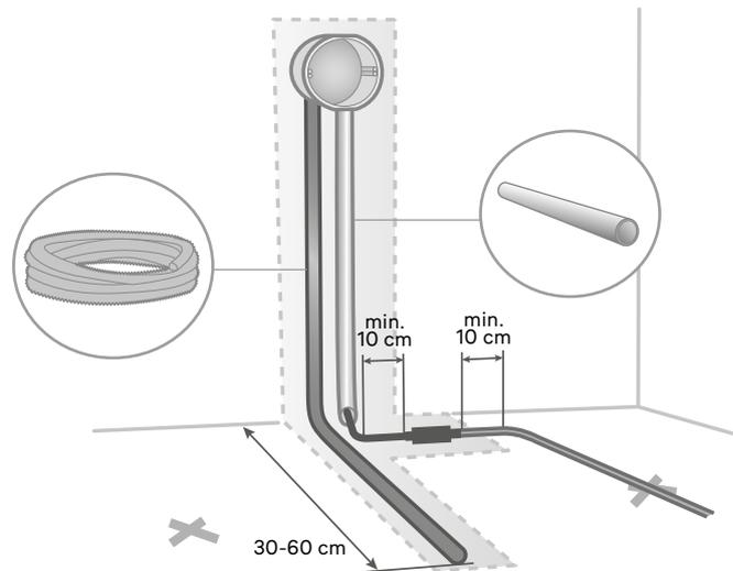
2a. The underfloor heating cable has a 2.5-metre connection cable. It is run in a VP tube/plastic tube designed for electrical materials.
