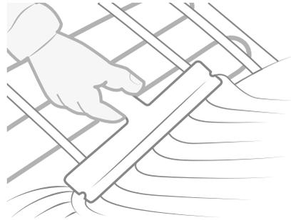
8. If possible, after applying screed, alternatively after flooring has been laid, perform a third insulation and resistance measurement of the heating cable. Fill in the test report or use Garantera on your smartphone.
