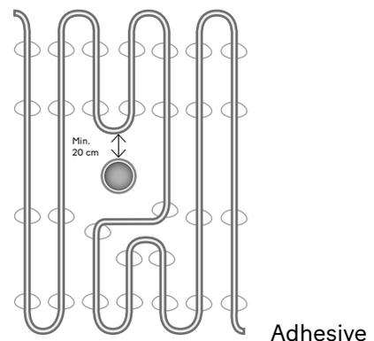
The cable may not be installed under fixed furnishings, such as toilet bowls. It can be advantageous to secure toilet bowls with silicone instead of screws.
