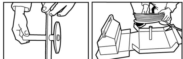
2. Perform the first insulation and resistance measurement of the cable. Fill in the test report or use Garantera on your smartphone.
