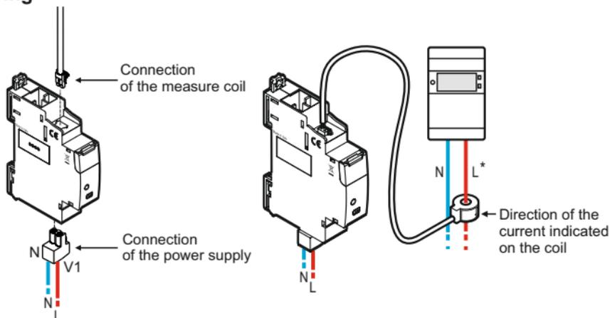
A circuit breaker with rated current C2 to C16 is necessary depending on wire section used for supplying the energy meter.
