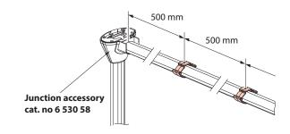
5.4 Fixing bracket cat. no 6 530 59 for Ovaline horizontal tube or Ovaline flexible horizontal kit
