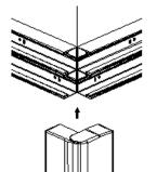
Positioning of the trunking to the wall before clipsage of the external angle
