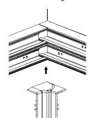
Positioning of the trunking to the wall before clipsage of the internal angle
