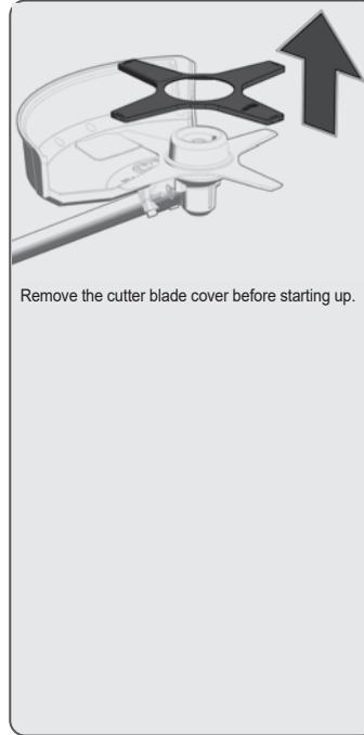
Remove the cutter blade cover before starting up.
