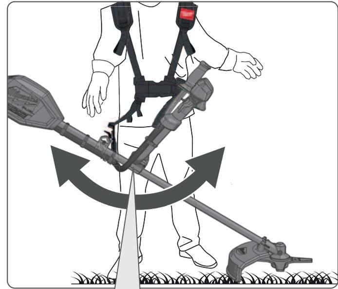
Level the appliance. The blade should touch lightly the ground.
