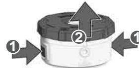
Discard any short line remnants. Snap the cover back onto the trimmer head.
