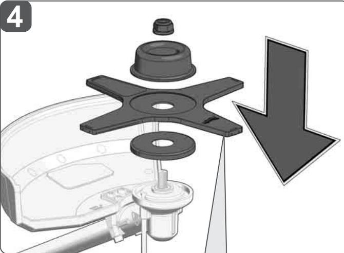
The blade can be used on both sides.
