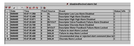
It is displayed by clicking the **disabled alarm list** button on the PCS 7 alarm logging status bar.
