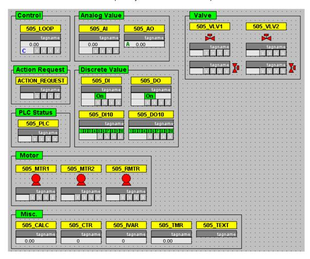
The 505 symbols are provided on picture "@@505Typicals.pdl". PCS 7/505 DBA uses these symbols as shown to create instances associated with the type found in the 505. The symbols on this picture can be considered "master" symbols. These symbols use a naming convention of @505\_Al/1. When DBA creates an instance of this symbol on a picture, the symbol name is set equal to the tagname of the 505 tag. DBA manages these symbol names and they should not be edited.
