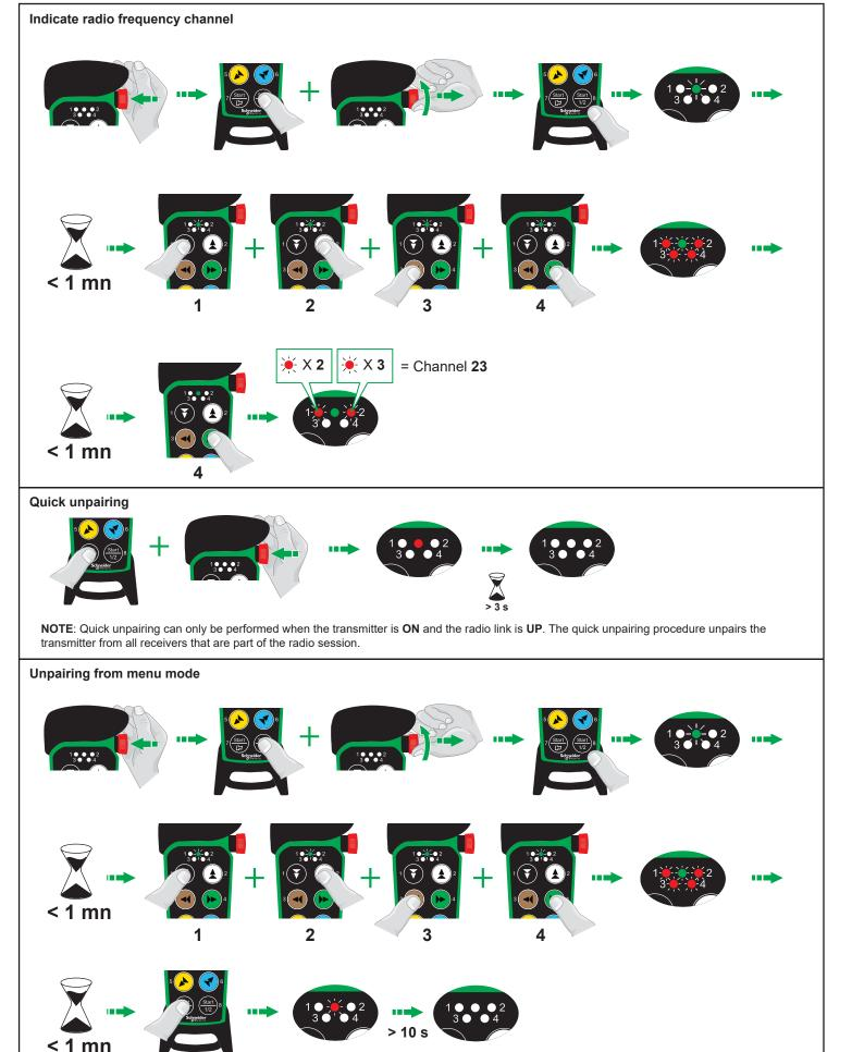
NOTE: This unpairing procedure can be used when the button 7 (used for quick unpairing) is used by another function.
