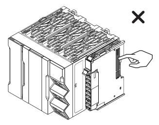
Do not write anything with ink within the restricted region of the CPU Unit that is shown in the following figure. Also do not get this area dirty. When the Unit is installed or removed, ink or dirt may adhere to the pins in the NX bus connector, which may result in malfunctions in the Unit.
