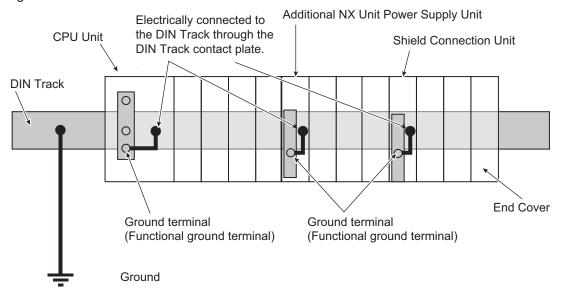
If the surface of the DIN Track is treated to produce an insulating material (e.g., anodized aluminum), the DIN Track contact plate will not be electrically connected to the DIN Track even if they are in physical contact.
