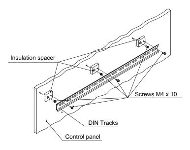
DIN Track Insulation Spacers NX-AUX01 (OMRON Corporation)
