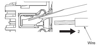
**3** Remove the flat-blade screwdriver from the release hole.
