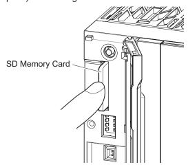
The SD Memory Card will be ejected from the compartment.
