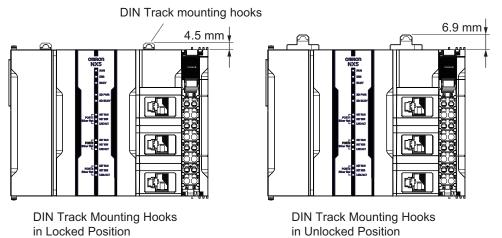
If the DIN Track mounting hooks are pulled up, they are in the unlocked position.
