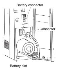
**4** Press in the battery harness by twisting and close the memory card cover.
