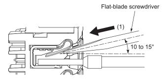
2. Leave the flat-blade screwdriver pressed into the release hole and tilt the flat-blade screwdriver approximately 5° to the direction of the ferrule.
