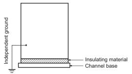
Example: Insulating and Grounding an Enclosure
