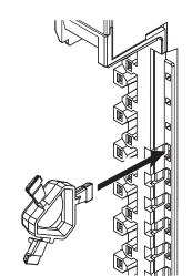
**2** Rotate the runner to break off the Coding Pin.
