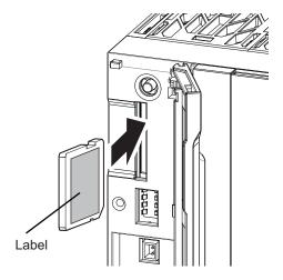
**3** Push the SD Memory Card securely into the compartment.
