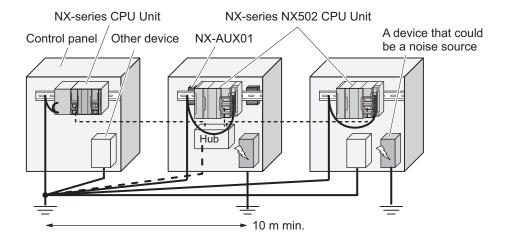
b. Installation method by connecting devices and noise sources to a common earth electrode This is an earthing method to connect the device that is connected with a communications cable, other devices, and a device that could be a noise source, to a common earth electrode. This earthing method is not recommended, because the device that is a potential noise source may interfere electromagnetically with other devices.
