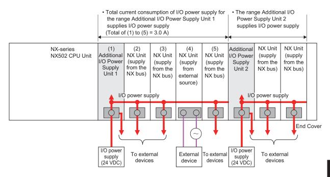
I/O power supply current consumption of each Unit
