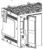
3 Connect the connector of the battery to the battery connector and insert the battery in the battery slot.
