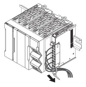
In such a case, secure wires within the range of 30 mm from the screwless clamping terminal block. Also, leave spaces below the CPU Rack to ensure ventilation, as shown in the following figure.
