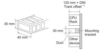
\*1. It varies depending on the DIN Track to be used. Refer to *Installation Dimensions* on page 5-32 under 5-3-14 Assembled Appearance and Dimensions on page 5-32 for details. It corresponds to the dimension (B).
