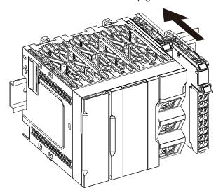
**3** Press the NX Unit with a certain amount of force against the DIN Track until you hear the DIN Track mounting hook lock into place.
