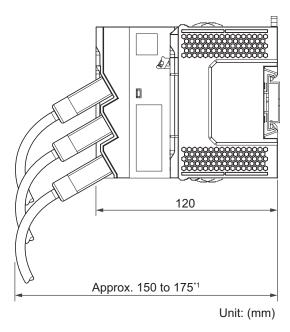
\*1. This is the dimension from the back of the Unit to the communications cables. Approx. 150 mm: When MPS588-C connector is used
