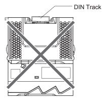
Mounting with the DIN Track Installed Vertically
