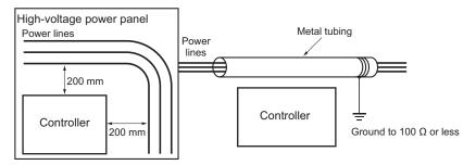
Example: Separating Controller from Power Lines
