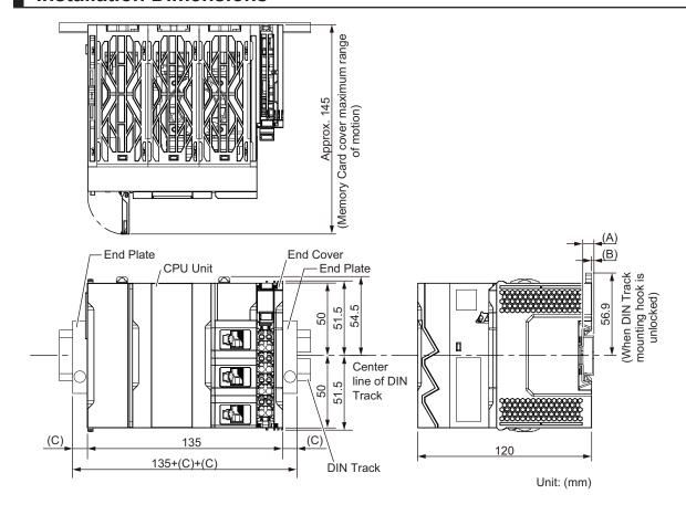
W: Width of CPU Unit (including the End Cover)
