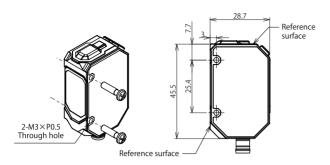
Mounting brackets are sold separately. Tightening torque for the mounting hole is 0.6 N·m or less (M3 screw).
