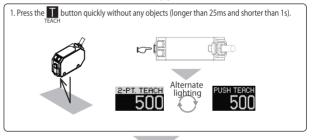
2. Press and hold the **T** button without any objects (longer than 1s and shorter than 5s). Release the button when [Reference (Normal)] is displayed on the display (Normal) • [Window FGS] is selected automatically as the output mode.
