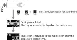
f buttons are operated in the key lock state, the key lock icon is displayed on the main screen.
