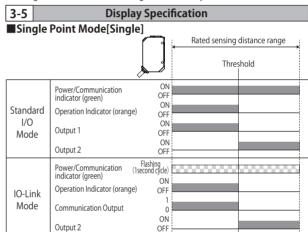
■Window BGS mode[Window BGS] Rated sensing distance range Near-side Far-side threshold threshold Power/Communication indicator (green) OFF Standard Operation Indicator (orange) OFF ON OFF 1/0 Output 1 Mode ON OFF Output 2 Flashing (1second cycle) Power/Communication indicator (green) Operation Indicator (orange) IO-Link OFF Mode Communication Output Output 2
