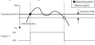
\*1. This is a graph when the output logic is N.O. It is inverted in the case of N.C.
