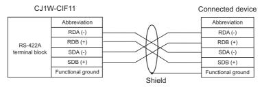
When connecting each of the signals with a twisted-pair cable, make the connections so that the RDA and RDB and the SDA and SDB become pairs of the twisted-pair cable. If the pair combinations are incorrect, a communication error may occur.
