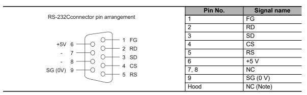
Note The hood will have the same electric potential as the connector hood of the connection destination.
