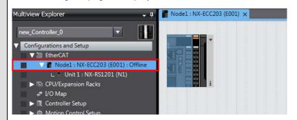
In the Edit Slave Terminal Configuration Tab Page, click your Load Cell Input Unit. The following tab page is displayed.
