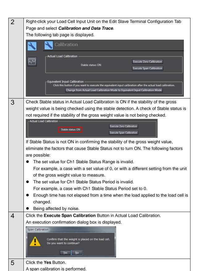
\*1. By default, the stable detection capability is disabled. Refer to *8-7 Stable Detection* described in the *NX-series Load Cell Input Unit User's Manual* (Cat. No. W565) for details on the stable detection feature.
