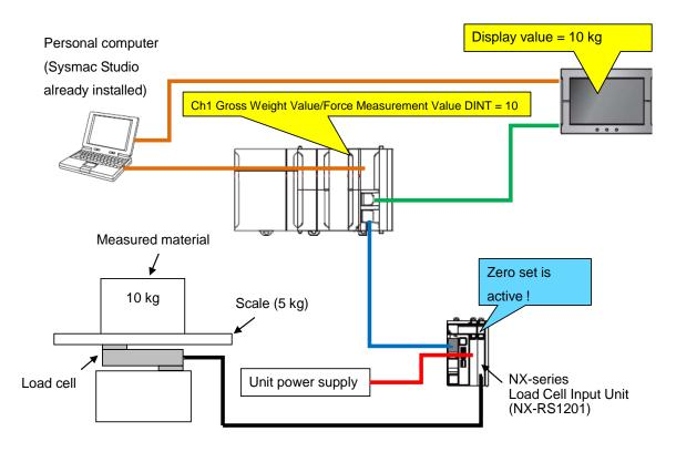
Refer to 8-3 Zero Set/Zero Reset described in the NX-series Load Cell Input Unit User's Manual (Cat. No. W565) for details on the zero set feature.
