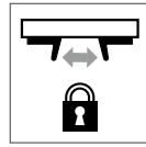
Before using the ladder, always make sure that the locking mechanism is in order and fully locked.
