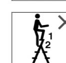
Never stand on the top two treads/rungs of a stepladder that does not have a platform and fittings for hands/knees to hold on to.
