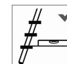
The treads of the hinged ladder must be horizontal
