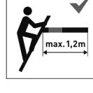
Ladder can be used in offset mode up to a maximum distance of 1.2 m.
