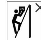
While using the ladder, do not carry heavy or bulky equipment.
