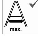
Only use the ladder when both ladder sections are fully secured and unfolded.
