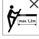
Support section in offset mode must be no longer than 1.2 m.
