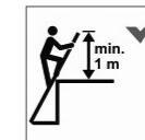
When using a single ladder to access greater heights, ensure that the ladder extends at least 1 m beyond the resting point and secure the ladder where necessary.
