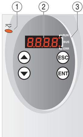
(1) Red LED on: voltage applied at DC bus
