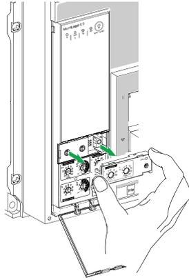
6. Inspect mounting area for debris and contamination.
