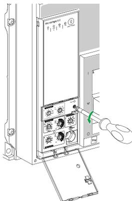
5. Remove the adjustable rating plug.
