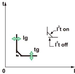
The ground-fault protection pickup  $I_g$  sets the level of ground-fault current at which the circuit breaker trips when reaching the ground-fault protection time delay  $t_g$ .
