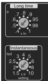
The instantaneous protection pickup  $I_{sd}$  is set by using the  $I_r$  and  $I_{sd}$  multi-position dials on the front face of the MicroLogic trip unit.
