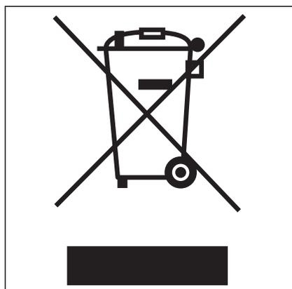
Electronic components and batteries must not be put in the domestic waste but must be disposed of appropriately in conformity with the WEEE guideline 2012/19/EU.
