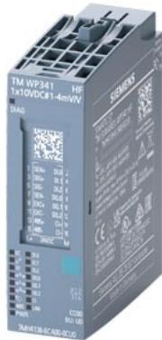
SIMATIC ET 200SP, TM SIWAREX WP341 HF, weighing module for conveyor belt scales and solids flowmeters, 3xDI, 3xDQ, 1xRS485, 1xEthernet, 1x LC (1-4mV/V)
