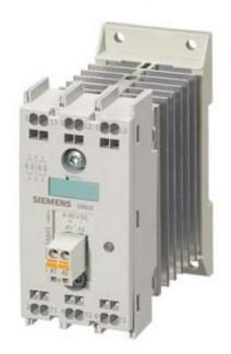
SEMI-CONDUCTOR CONTAC.3-PH.3RF2 AC51 10A 40 DEG. C 48-600V / 4-30V DC 3-PHASE CONTROLLED SPRING-LOADED CONNECTION BLOCKING VOLTAGE 1200V
