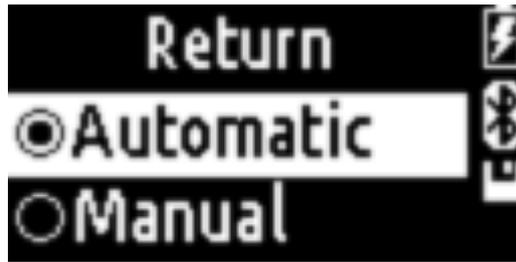
Figure 11. End of measure automatic return mode setting screen.
