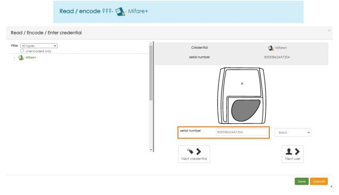
The serial number will be recorded and a blue pop-up window will be displayed at the top confirming the encryption. Once encoded, press Save .
