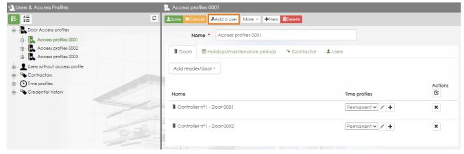
This will allow the user(s) to be generated to access the doors enabled in profile 0001 (door 01 and door 02).
