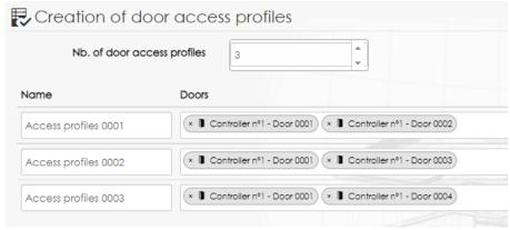
For example, in the capture all profiles can access "door 01" which could be a general access door common to all users, while the second door of each profile is a specific one. These could be for example for access to floor 2, floor 3 and floor 4.
