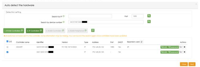
Select the rest of the detected IP controllers  $\checkmark$  and press  $\overset{\text{Next}}{}$ .
