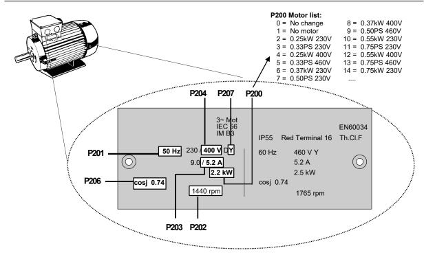
Figure 5: Motor type plate
