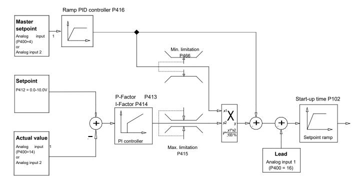
Figure 8: Process controller flow diagram
