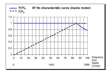
Figure 15: 87 Hz characteristic curve
