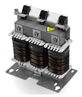
An output choke should be fitted for low powers up to 370 kW, for motor cable lengths over 50 m / 15 m (unshielded / shielded) and for higher powers for motor cable lengths over 100 m / 30 m (unshielded / shielded). All chokes have a protection class corresponding to IP00. The choke used must therefore be installed in a control cabinet.
