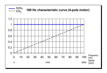
Figure 16: 100 Hz characteristic curve
