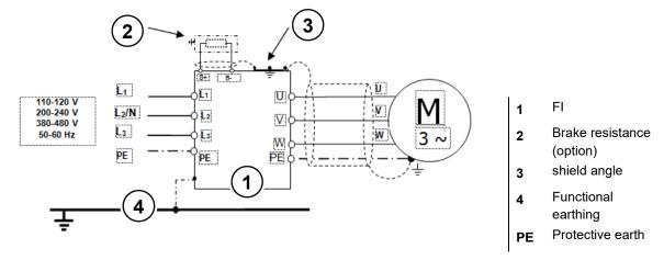
Figure 9: Wiring recommendation
