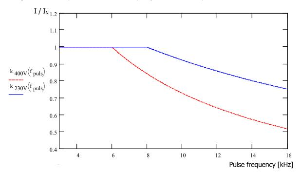
Figure 10: Heat losses due to pulse frequency
