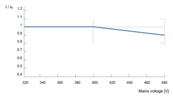
Figure 11: Reduced output current due to low voltage
