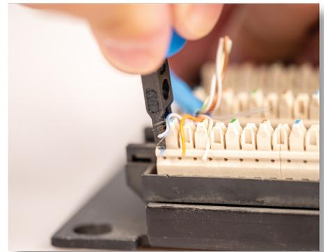
Designed as an economical option for seating and trimming wire in 110 type punchdown blocks, the PD-110 is perfect for small do-it-yourself jobs on 110-terminal blocks. This non-impact punchdown tool features the following:
