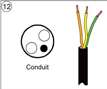
12. Connect the grounding conductor to the grounding terminal (12a) and the other conductors to the R+ and R- terminals (12b). Tighten the screws to the torque given in the table.
