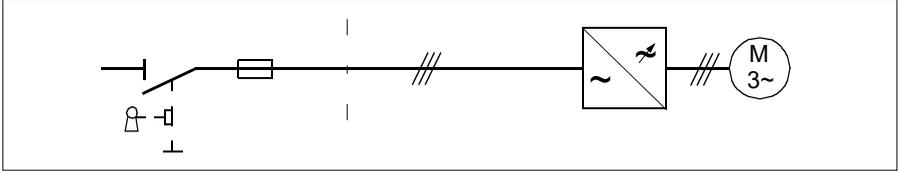
Size the fuses at the distribution board according to instructions given in chapter [Technical data](#), page 268. The fuses will protect the input cable in short-circuit situations, restrict drive damage and prevent damage to adjoining equipment in case of a short-circuit inside the drive.
