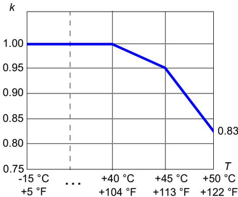
**-414A-4 and -430A-4:** In the temperature range +35...40 °C (+95...104 °F), the rated output current is derated by 3.2% for every added 1 °C (1.8 °F). In the temperature range +40...45°C (+104...113°F), the rated output current is derated by 0.85% for every added 1 °C (1.8 °F). In the temperature range +45...50 °C (+104...122 °F), the rated output current is derated by 2.2% for every added 1 °C (1.8 °F). The output
