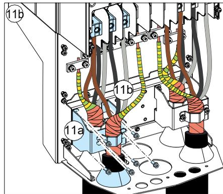
12. Install the grounding shelf of the control cables.
