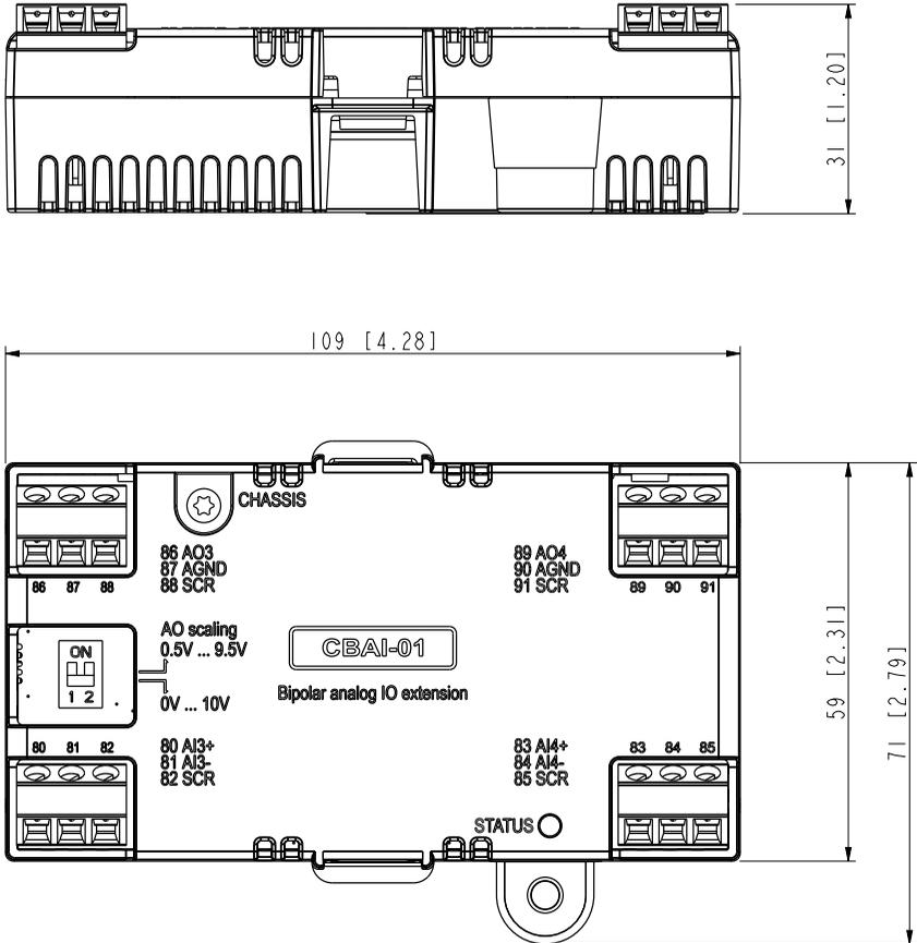
**Installation:** Into an option slot on the drive control board
