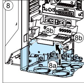
**Note:** Install the hood to UL Type 12 drives after you have installed the drive electrically and reinstalled covers, see page [224](#).
