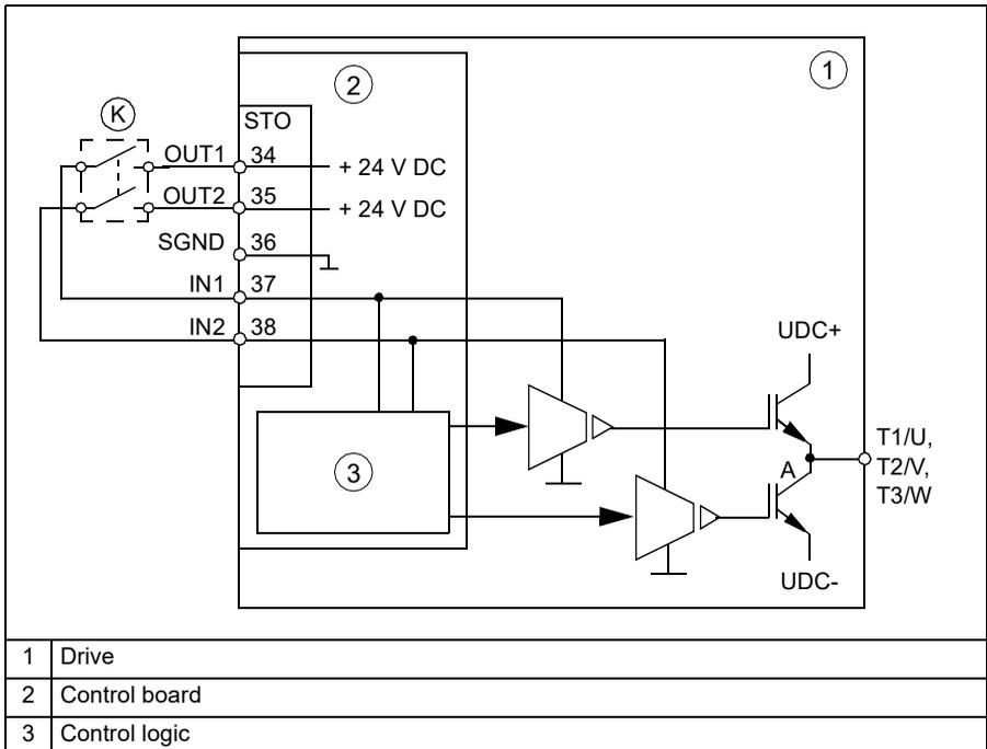
An example of a Safe torque off wiring is shown below.
