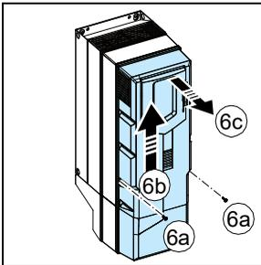
**Note:** Install the hood for UL Type 12 drives after you have installed the drive electrically and reinstalled covers, see page 224.
