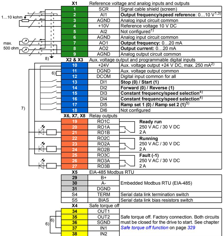
Total load capacity of the Auxiliary voltage output +24V (X2:10) is 6.0 W (250 mA / 24 V DC). Digital inputs DI1...DI5 also support 10 to 24 V AC.
