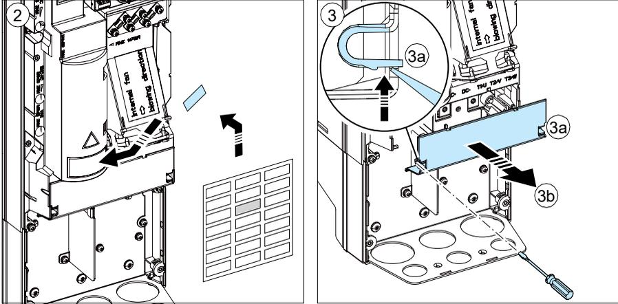
4. Remove the rubber grommets, if present, for the motor and input power cabling. Remove the grommets for the control cabling when you are connecting them.
