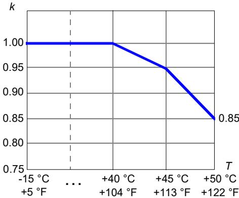
**-260A-4, -293A-4 -361A-4 and -363A-4:** In the temperature range +40...45 °C (+104...113 °F), the rated output current is derated by 1% for every added 1 °C (1.8 °F). In the temperature range +45...50 °C (+113...122 °F), the rated output current is derated by 2.5% for every added 1 °C (1.8 °F). The output current can be calculated by multiplying the current given in the rating table by the derating factor (k):
