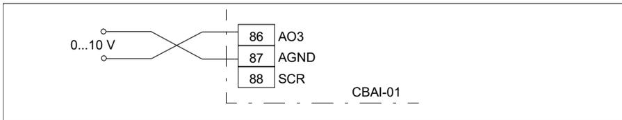
An alternative way to make the connection is to connect the cable shield to the SCR terminal of the control board.
