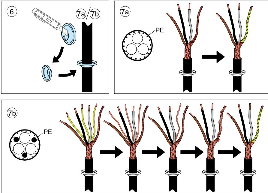
8. Slide the cables through the holes in the cable entry and attach the grommets to the holes (the motor cable to the right and the input power cable to the left).
