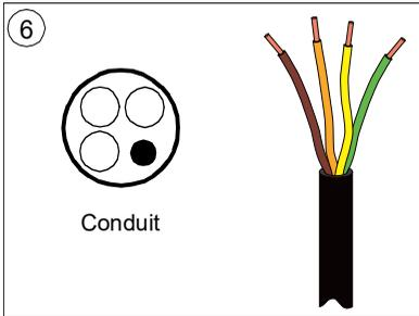
7. Slide the conductors through the conduit.
