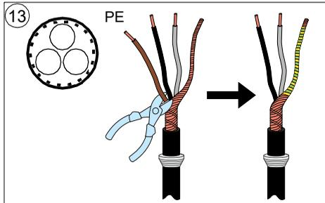
14. Connect the cable as the motor cable in step 7. Ground the shield 360 degrees (14a). Connect the twisted shield to the grounding terminal (14b) and the conductors to the R+ and R- terminals (14c) and tighten to the torque given in the table.
