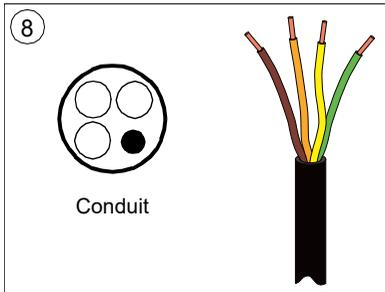
9. Slide the conductors through the conduit.
