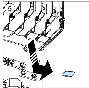
6. Remove the rubber grommets, if present, for the motor and input power cabling. Remove the grommets for the control cabling when you are connecting them.
