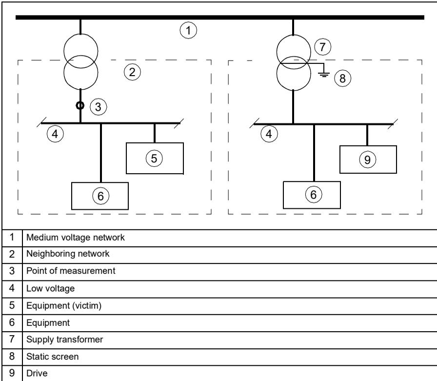
2. An EMC plan for preventing disturbances is drawn up for the installation. A template is available from the local ABB representative.
