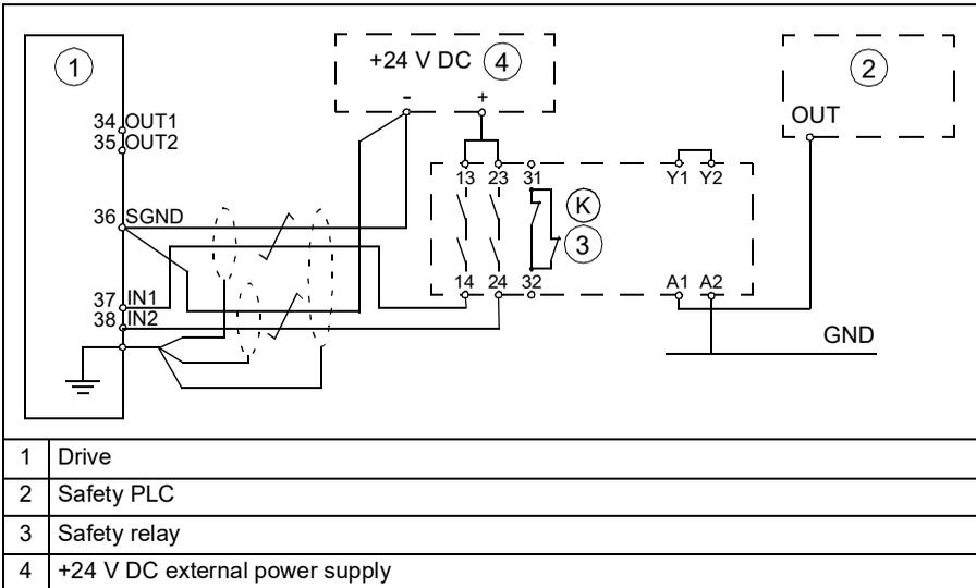
■ Multiple ACS580-01 drives, internal +24 V DC power supply
