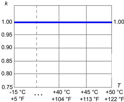
■ Ambient temperature derating, IP55 (UL Type 12)
