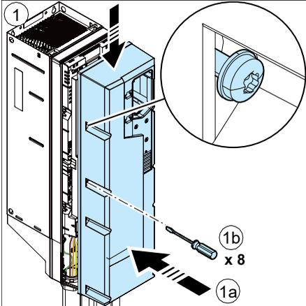
■ Reinstalling side plates and covers, frames R6...R9
