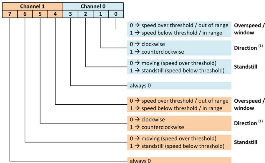
(1) Direction is only indicated if encoders are used. The value of the bit is of no relevance if only proximity sensors are used.
