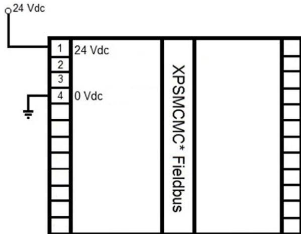
**NOTE:** Best practice dictates the use of fusing on the incoming 24 Vdc power, and sized appropriately for the requirements of the module.
