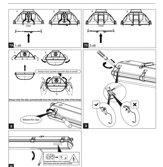
The light source in this luminaire may be replaced only by the manufacturer or its contractual service technician or a similarly qualified person!
