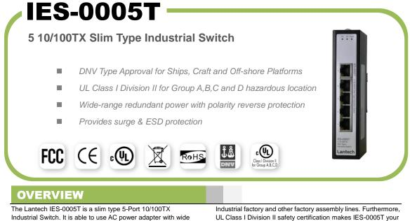
The Lantech IES-0005T is a slim type 5-Port 10/100TX Industrial Switch. It is able to use AC power adapter with wide DC input range and can be installed easily with DIN rail or wall mount kit.
