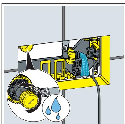
➤ Open the corner valve for a few seconds to flush the pipe.
