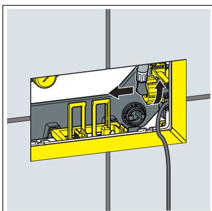
➤ Loosen the flexible hose at the filling valve.
