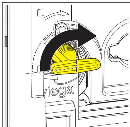
► Turn the retaining bolts by 90° in a clockwise direction.
